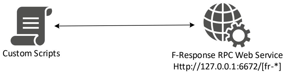
F-Response uses JSON POST style communication between the script and a localhost bound webservice on the examiner machine to perform commands and receive responses.
